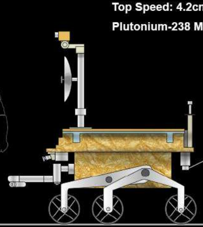
Yutu (2013/2019) 1.5m x 1.1m x 1.1m 140kg Top Speed: 5cm/s Plutonium-238 RHUs
